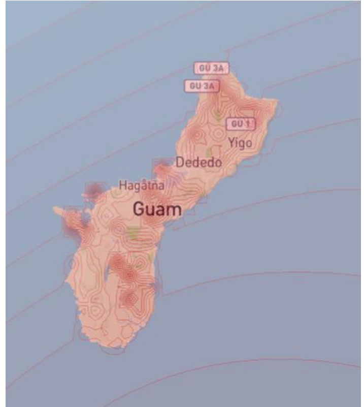
Figure 8: Resulting peak ground acceleration (PGA) from the 7.8Mw earthquake. Image from FRONTIER.
